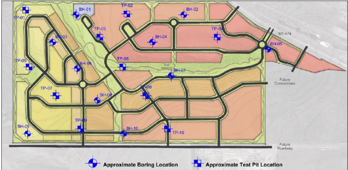
Figure 5. Test Pit Locations
